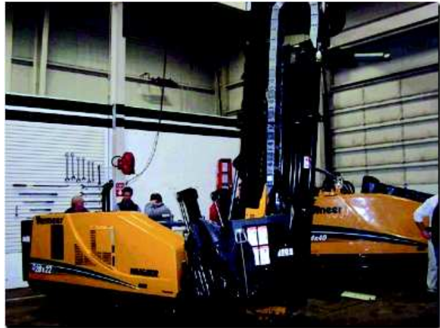
The new D20X22FX Series II Flex Drill from Vermeer is capable of entry points from 18 to 90 degrees, doing the work of two machines.
