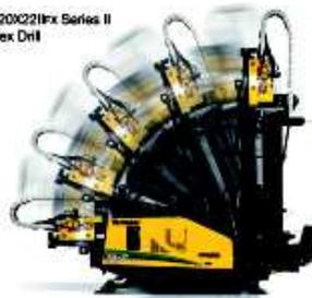
Inspired by the voice of drillers and fueled by the Vermeer passion for innovative solutions, the Vermeer® D20x22Flex Series II Navigator® flex-angle drill is the industry's first drill capable of entry points from 18 to 90 degrees - and everywhere in between.
